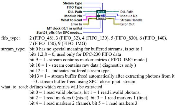
The procedure is needed to initiate the process of extracting photons from a stream of photons placed into PC memory buffers previously 'buffered' stream.
