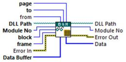
The procedure reads data from a block of the SPC memory (on module 'mod\_no') defined by the parameters 'block', 'frame' and 'page' to the buffer 'data'. The procedure is used to read measurement results from the SPC memory especially for SPC7x0/830/140/15x/160 modules in scanning modes ( when frames per page is greater than 1).
